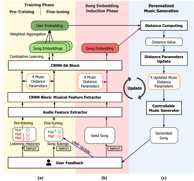
Figure 1: Workflow of the UMP Extraction and Personalized Music Generation System. (a) Training Phases of the UMP Embedding Model. (b) Process of Computing the Embedding of an Input Seed Song. (c) Process of Personalized Music Generation.
