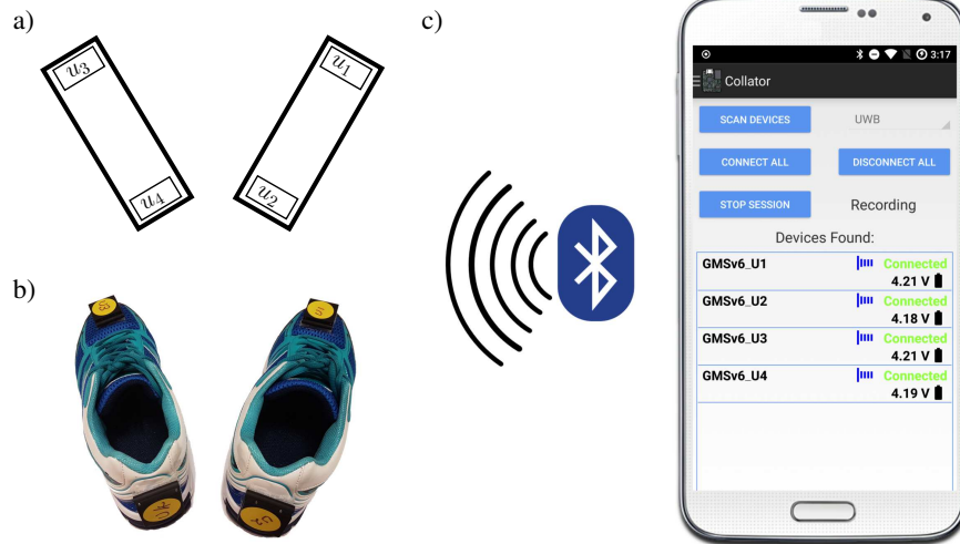
Fig. 3. Components of the system: Shoe sensors, and linked smartphone application.
